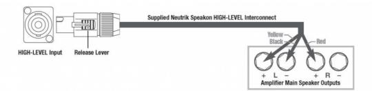
For differential (i.e. fully balanced) amplifiers using one REL, simply use the standard connecting scheme with the exception of connecting the black wire to chassis ground (i.e. a metal bolt or screw, preferably not painted or anodized, on the chassis of the power amp or receiver), not to a negative speaker terminal, and then connecting into the HIGH-LEVEL INPUT on the REL.
